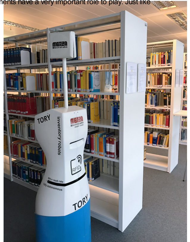
The Tory robot uses radio frequency identification technology to track inventory levels.
